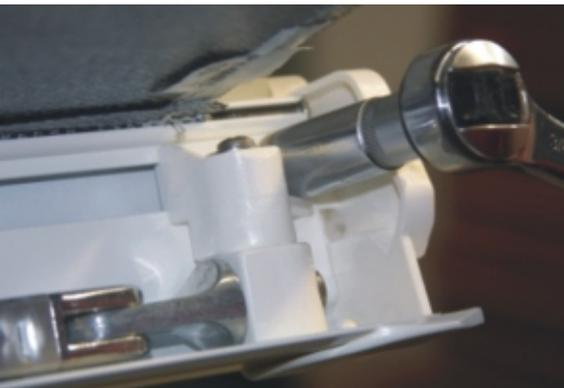
**2.-** Open the lead bar and using a 13mm wrench loosen the bolt and remove the lead bar cap.
